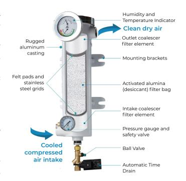
air moves upward through a felt pad, and after through the desiccant bag which attracts and absorbs the moisture from the air before it flows through another series of felt pad and coalescer element.
