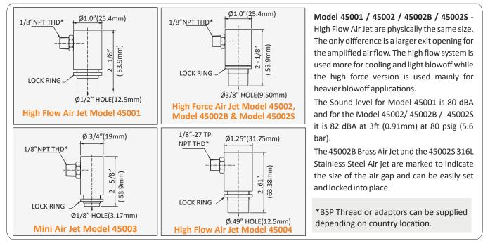
Air Jets perform similar to Adjustable Air Amplifiers - with the same lock ring and methodology. **Nex Flow**<sup>®</sup> Air Jets are adjustable and come with a lock ring to fix the gap.
