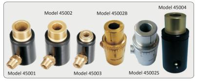
The **Mini Air Jet Model 45003** is ideal for small spots where a Nozzle may not be adequate for wider coverage of air flow. It is most compact air jet available with high force and adjustability. Sound level is 82 dBA at 3ft (0.91mm) at 80 psig (5.6 bar).
