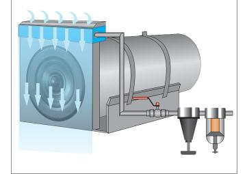
Two Model 10012 Standard Air Blade® Air Knives are installed on a duct (One on top, One on bottom) to draw in waste fumes & exhaust. The air leaving the Air Knives hug the inside wall creating an excellent vacuum inside the duct.
