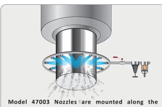
Model 47003 Nozzles are mounted along the circumference of a one meter diameter piston rod to blow off debris from its surface. The Nozzles are operated only when piston rod retracts in to the cylinder.
