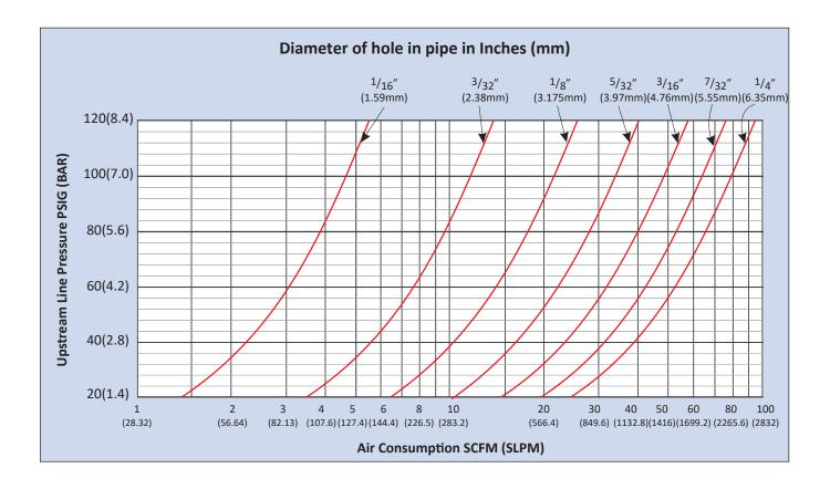
Open tubes and pipe create a great deal of noise due to the energy loss from turbulent flow. Not only is there a great deal of compressed air used, the flow is mostly turbulent so the force required for many blow off applications can dissipate quickly and become weak after only a few inches from the opening.
