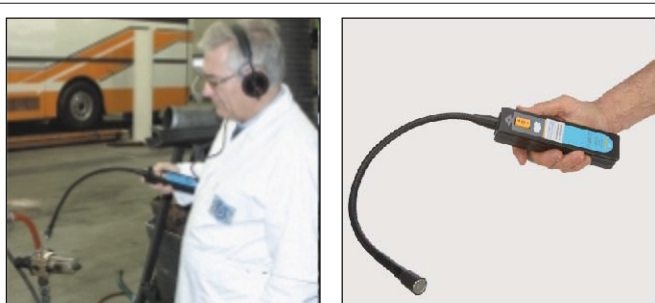
Above shows use of quality headphones and flexible pipe with sensor to get to a difficult spot to find an air leak.
