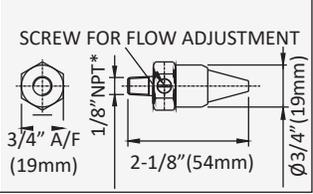
SCREW FOR FLOW ADJUSTMENT
