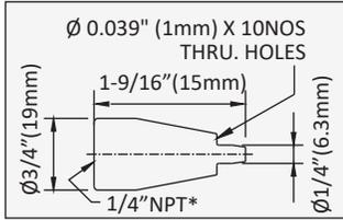
**Model 47010** - Is a unique design by Nex Flow® and is extremely powerful. It has a 1/4" female NPT fitting and is fully anodized for long life. With the 'coanda' profile you get an extremely strong force at a distance. This is an ideal Nozzle for blow guns and for blowing small parts for part ejection heavier viscosity liquids. The 47010 is a higher force Nozzle but has less distance for laminar flow than the 47004. Use the Model 47004 is greater distance required from the Nozzle.
