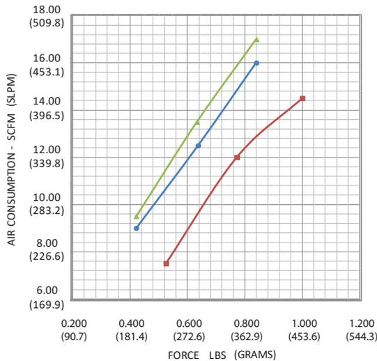
**FORCE EFFICIENCY OF THE NEX FLOW® MODEL 47004AMF AIR MAG® NOZZLE TO COMPETITIVE VERSIONS**
