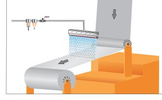
A Model 16118X removes static from extruded rubber web on a rewind. Previously the static charge was so high that any spark would cause the rubber to burn which regularly happens the 'extra strong' VS Bar combined with the X-stream<sup>®</sup>Air Blade<sup>®</sup> eliminated this unsafe situation.
