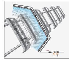
Three 24" X-Stream®Air Blade® lonizers Blow off dust from Automotive Bumpers prior to painting. The NEX FLOW® PLCFC controls the air on and off as required minimizing air consumption. In this case the static bars were "daisy-chained" together minimizing extraneous cable and reducing the number of power supplies needed.
